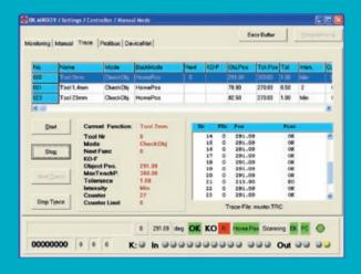
The easy to use Windows based software was developed specifically for the BK Mikro controllers and is used for the initial controller setup and to make any subsequent parameter adjustments. It also displays the current scanning results, any error messages, views the 32 previously stored faults, and saves/restores settings from a file. The connection to the PC is done using a standard mini-B 5 pin USB cable.
